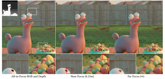
Fig. 8. Artifacts at large depth discontinuities. We present simulation results of a scene with a large depth discontinuity near the face of the toy. The red boxes indicate regions of large depth discontinuities where artifacts are visible. (Credits: “The Daily Dweebs” 3D scene courtesy of Blender Studio and Hjalti Hjalmarsson)
