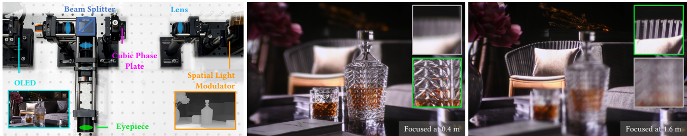
Figure 1: Left : Our display prototype. Middle and Right : Captured images from our prototype using a Nikon Z5 with a near (mid) and far (right) camera focus, at F/5.6 , 100 ISO, and 1.3 sec exposure. (Scene courtesy of “Entity Designer” at Blender Market)
